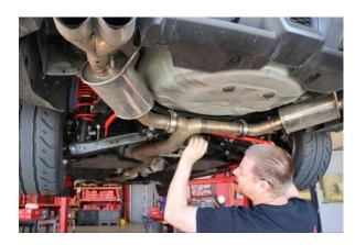
Step 4. Apply the supplied grease to the inside of the Eibach sway bar bushings. Install left and right sway bar bushings on the Eibach sway bar to the outside of the locating rings. Install the Eibach rear sway bar in the vehicle.
