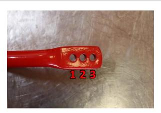
Step 6. Install left and right upper sway bar end links in one of the holes provided in the Eibach sway bar. Position 1 will provide the stiffest setting, position 3 will provide the softest setting. Install the left and right upper sway bar end link nut and tighten to factory specification. Lower vehicle and test drive listening for any abnormal noise.
