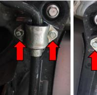
Step 2. Remove the four rear sway bar bracket bolts and remove the left and right rear sway bar brackets.
