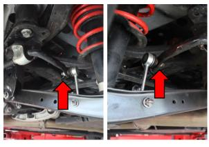
Step 1. Lift the rear of the vehicle using a suitable jack or lift to gain access to the rear way bar. Note: Never work on or under a vehicle unless it is properly supported by safety stands and wheels are blocked. Remove the left and right upper sway bar end link nuts.
