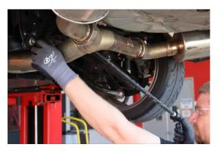
Step 3. Remove the sway bar from the vehicle.
